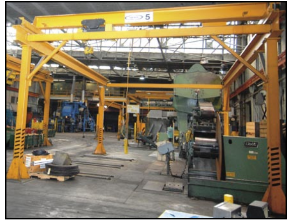
NELSON 5 ton free standing crane system
