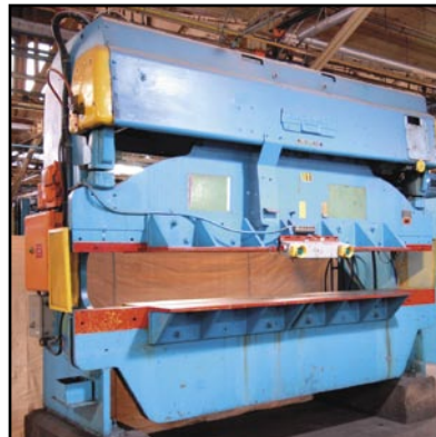
WYSONG 10' x 16 ga. mechanical shear
