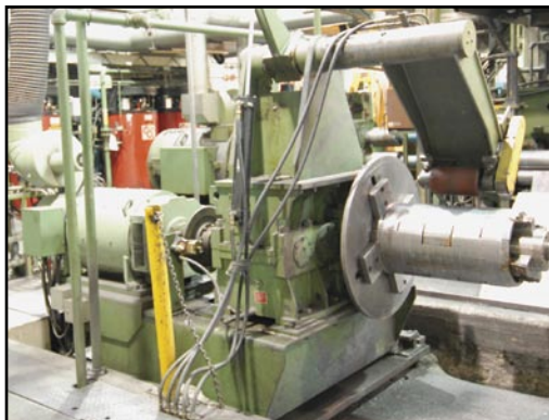
Rewriter with belt wrapper and pushoff
