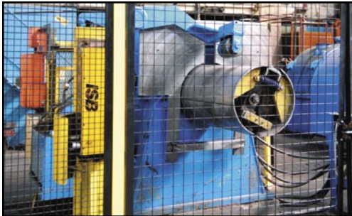
(2) custom built strip levelers on common base
