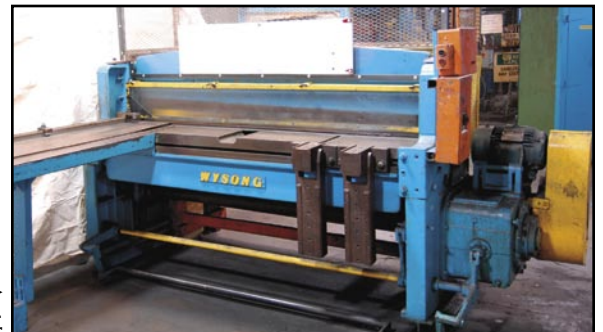
HAUSEN 10' x 16 ga. mechanical shear
