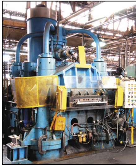
WEAN UNITED 1,500 ton hydraulic inflation press
