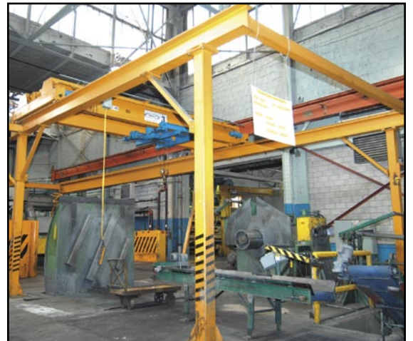
NELSON 3 ton free standing crane system
