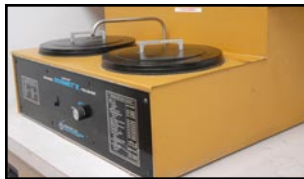
BUEHLER V grinder/polisher
