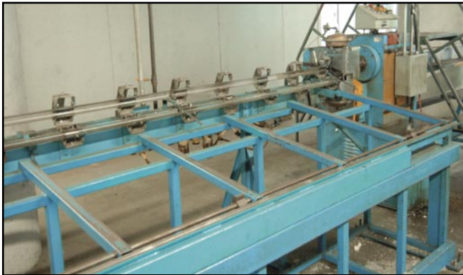
VENABLES Starfin strip opener & winder
