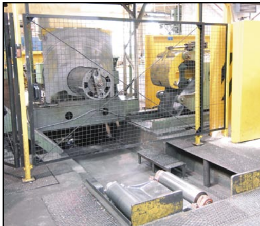
Rewriter with belt wrapper and pushoff
