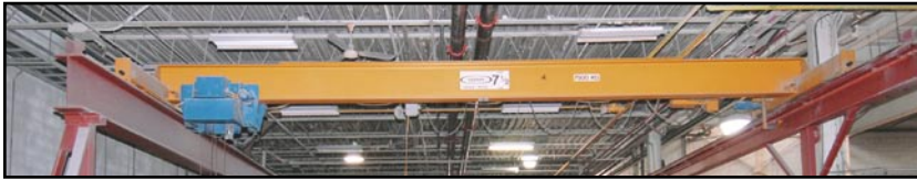
NELSON 7.5 ton free standing crane system
