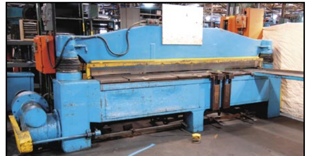
HAUSEN 10' x 16 ga. mechanical shear
