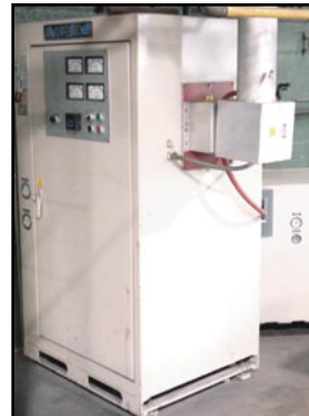
LEPEL induction heating power
