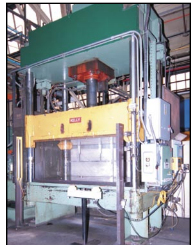
KELLY 300 ton four post hydraulic press
