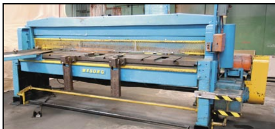
WYSONG 10' x 16 ga. mechanical shear
