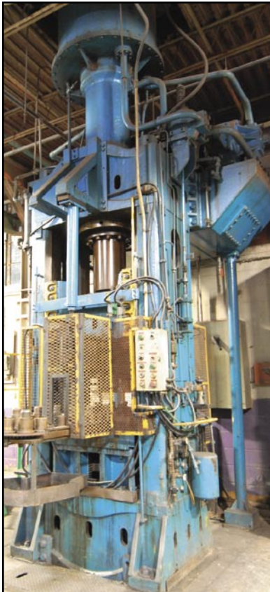
DOMINION 200 ton hydraulic press w/vertical necking fixture
