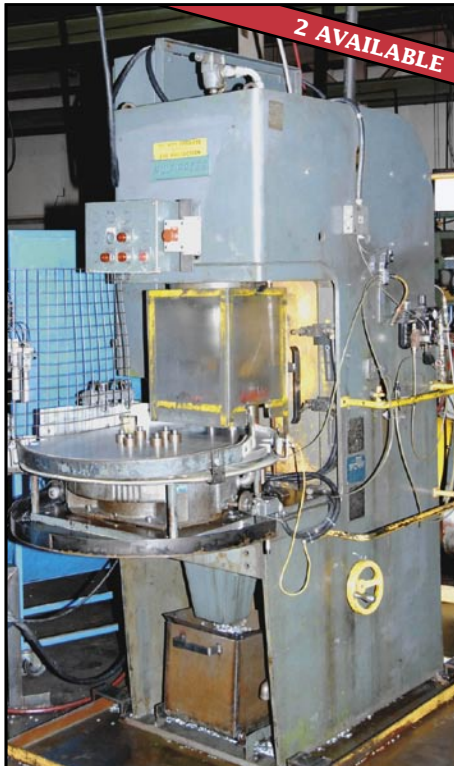
DENNISON 20 ton C frame hydraulic press with 6 position rotary index table
