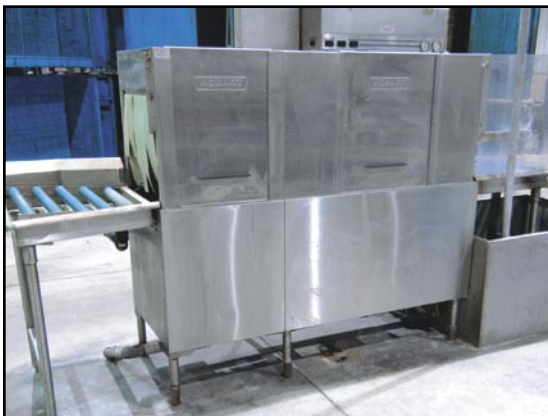
HOBART CRS 66AW 2 stage stainless steel parts washer
