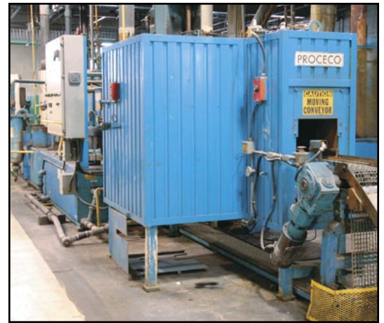
PROCECO BCW 12X12-4W-2R-8D-G-B 3 stage, parts washer
