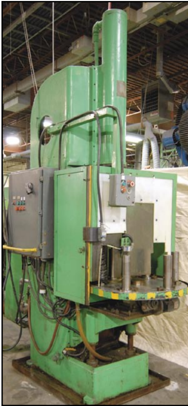
AMERICAN 12 ton hydraulic C frame press with 6 station rotary table
