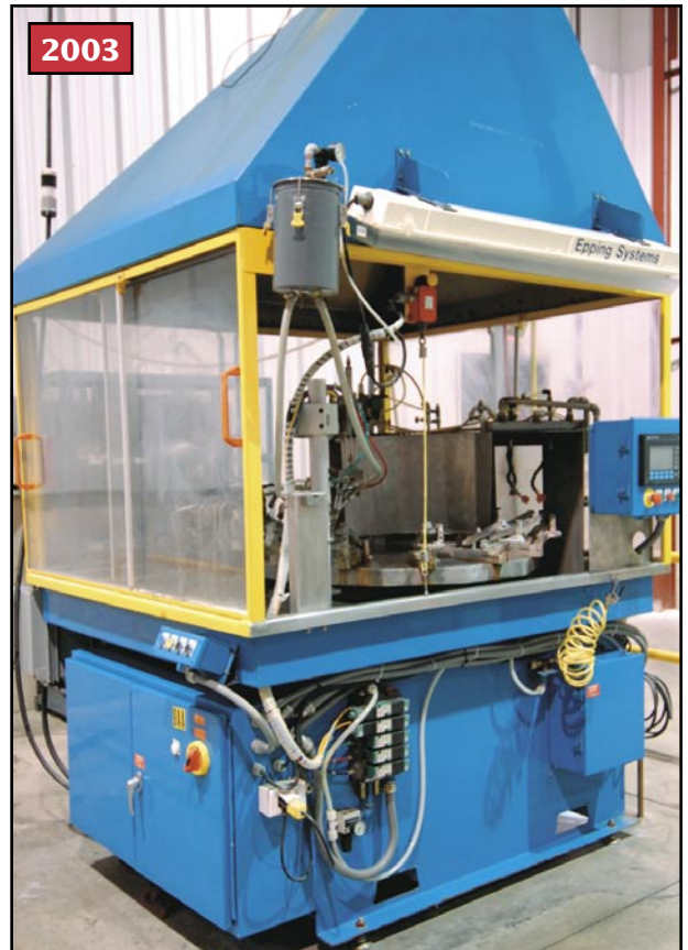
INDUSTRIAL COMBUSTION SOLUTIONS BS250 gas fired, 12 station rotary brazing system
