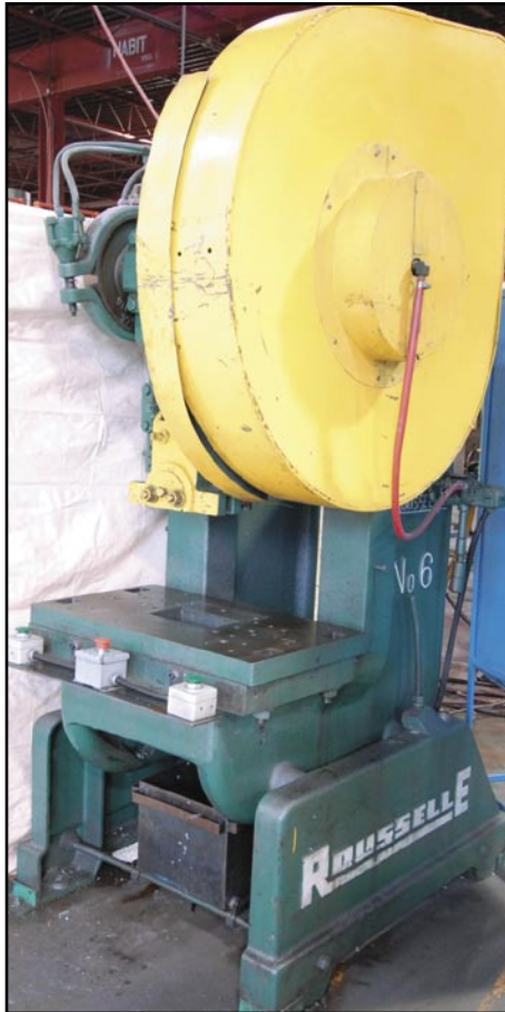
ROUSSELLE 60 ton flywheel type OBI press with air clutch
