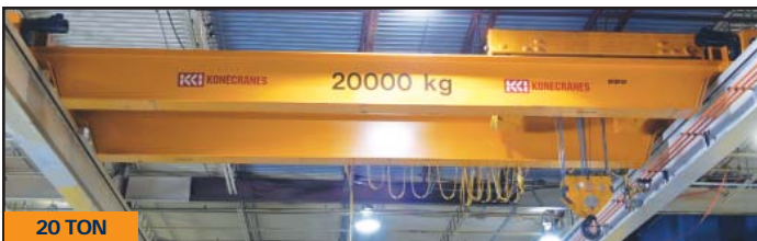
20 TON KONE 20 ton double girder top running bridge crane
