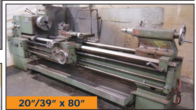
TOS SN63B gap bed engine lathe
