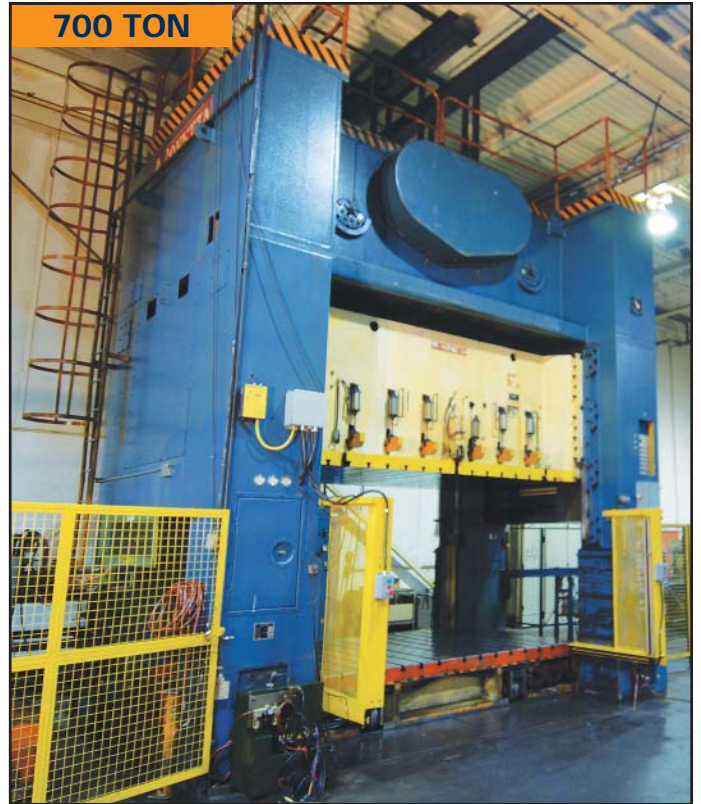
ROVETTA S4-700-132-84 700 straight side 4 point press
