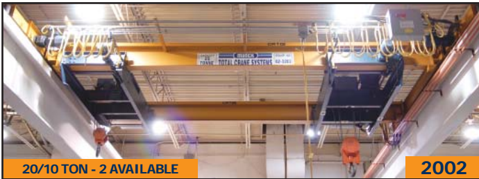
20/10 TON - 2 AVAILABLE 2002 MUNCK 20/10 ton double girder top running bridge crane
