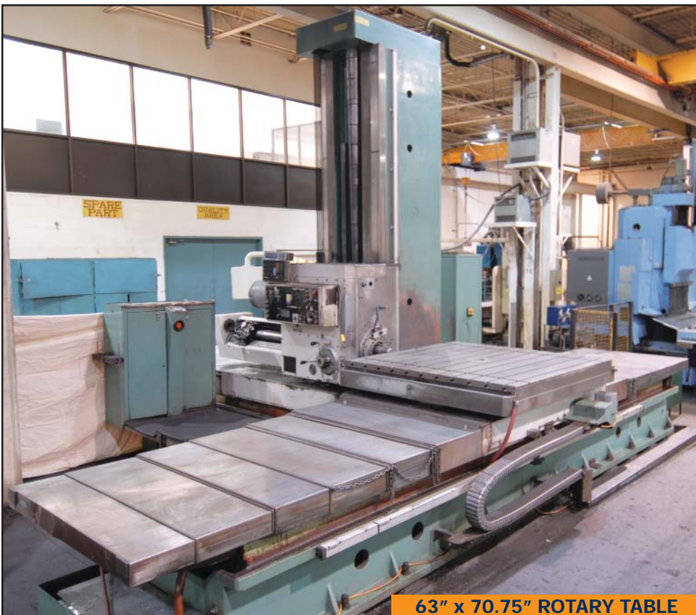
TOS WHN138A 5" table type horizontal boring mill
