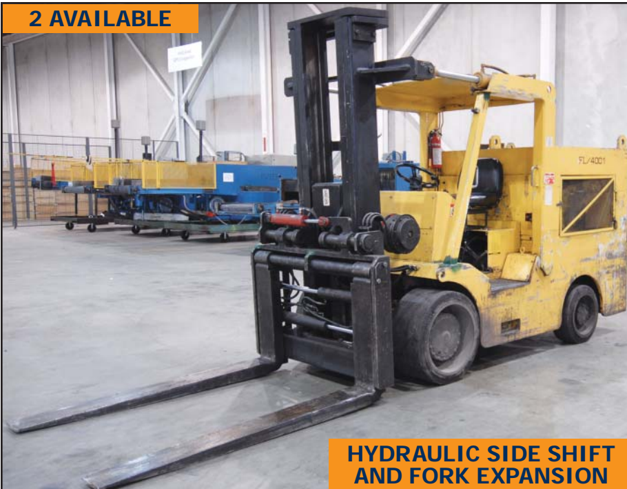
APACHE MA400AHT 40,000 lb capacity LPG forklift
