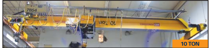
10 TON KONE 10 ton single girder underslung bridge crane
