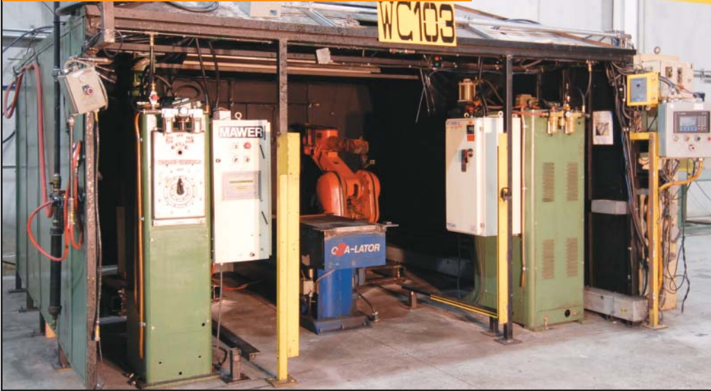
AUTODYNE dual robotic MIG welding cell
