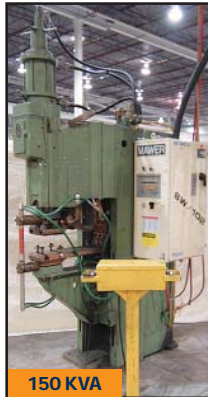
150 KVA TAYLOR WINFIELD ERB-18 spot welder
