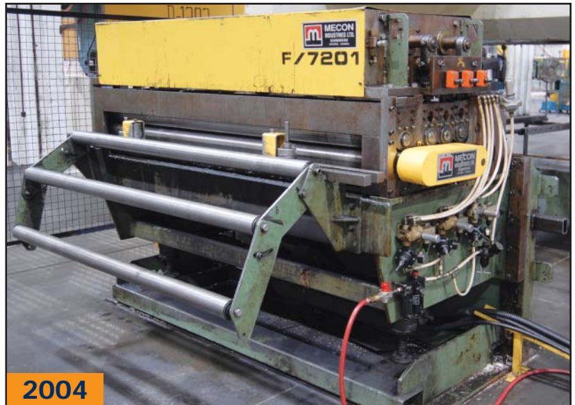
MECON 500FSP721 72" servo feeder
