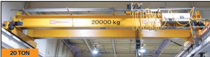
20 TON KONE 20 ton double girder top running bridge crane
