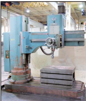
MAS VR5A 5' way type radial arm drill
