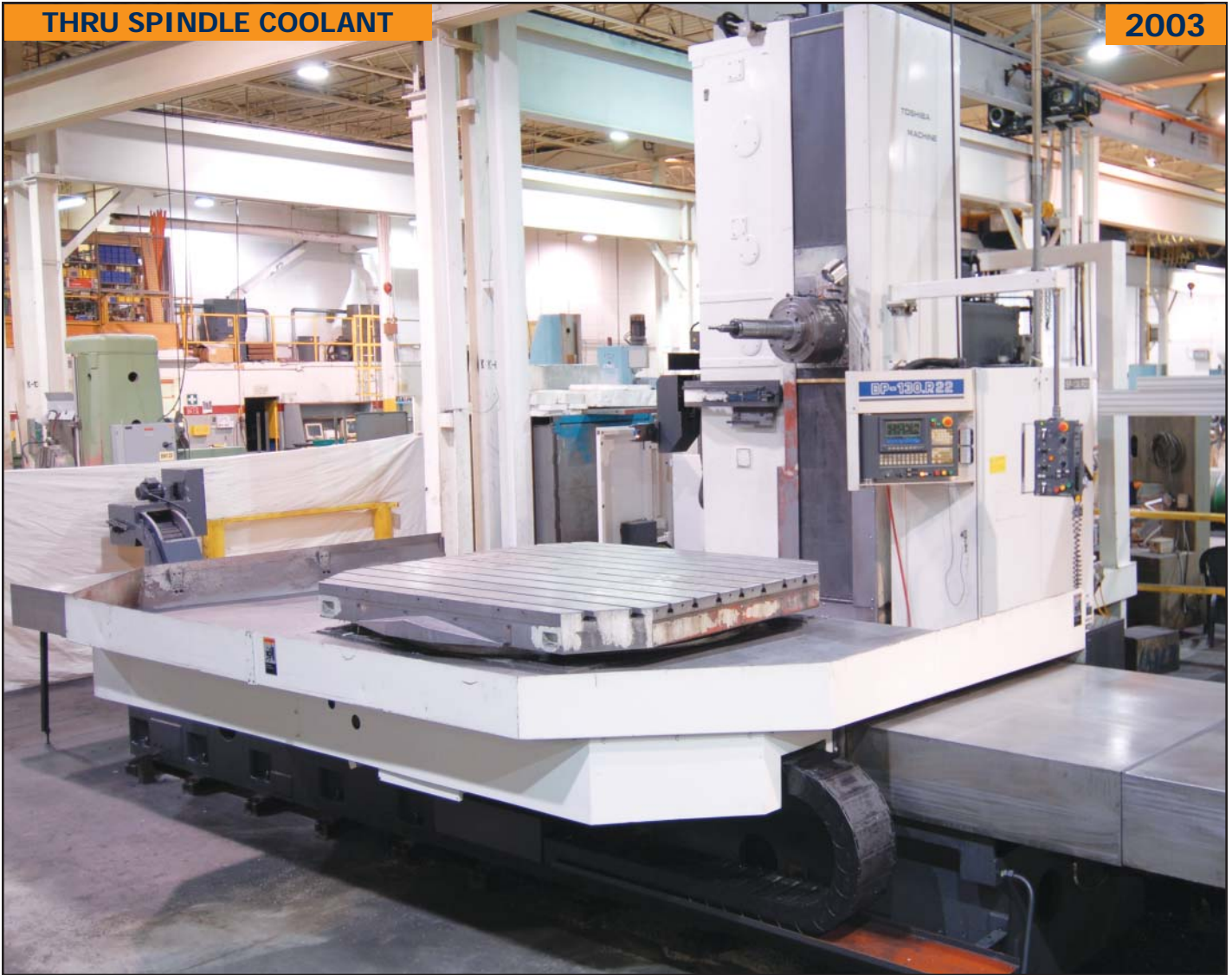
TOSHIBA SHIBAURA BP-130-R22 5.1" CNC table type HBM
