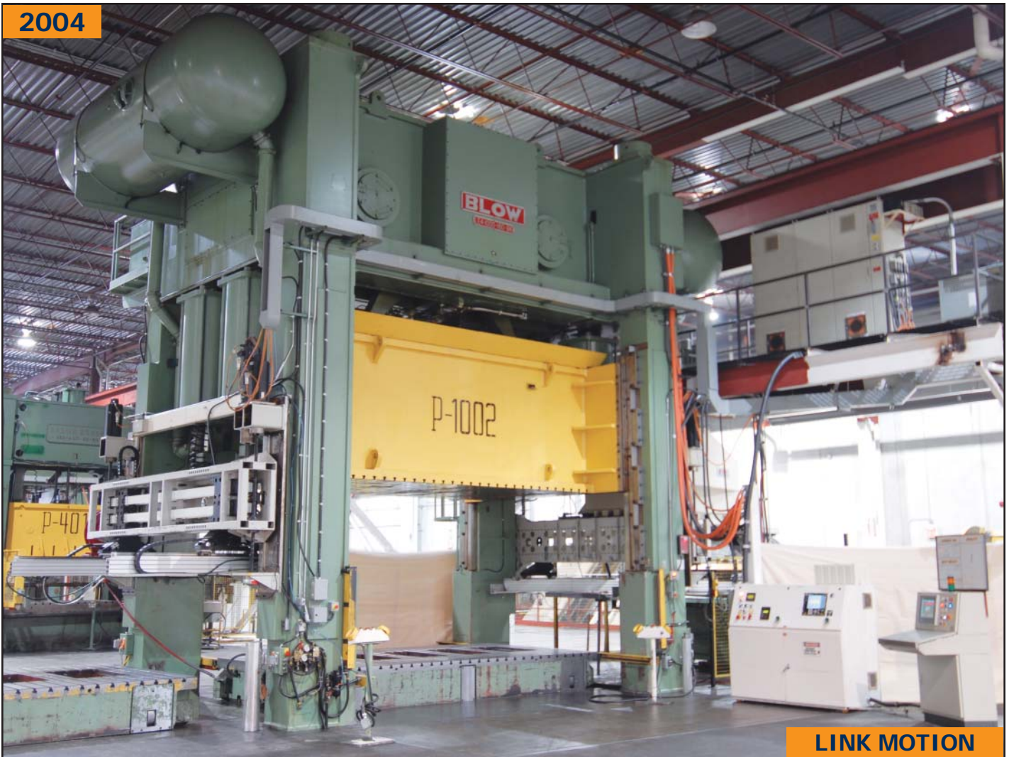
BLOW LE4-1000-180-96, straight side 4 point link motion press
