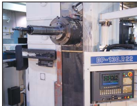
View of 5.1" spindle and TOSNUC 888 CNC control
