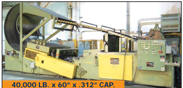
FEED LEASE FLCCD-6072-P40 coil cradle/straightener
