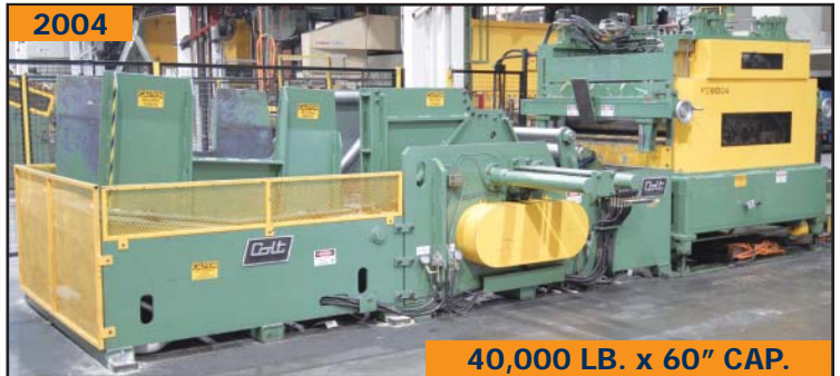
COLT SPACESAVER CSS-4000-60 integrated servo feed line
