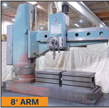
MAS VR8A way type radial arm drill
