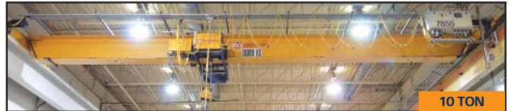
10 TON KONE 10 ton single girder underslung bridge crane
