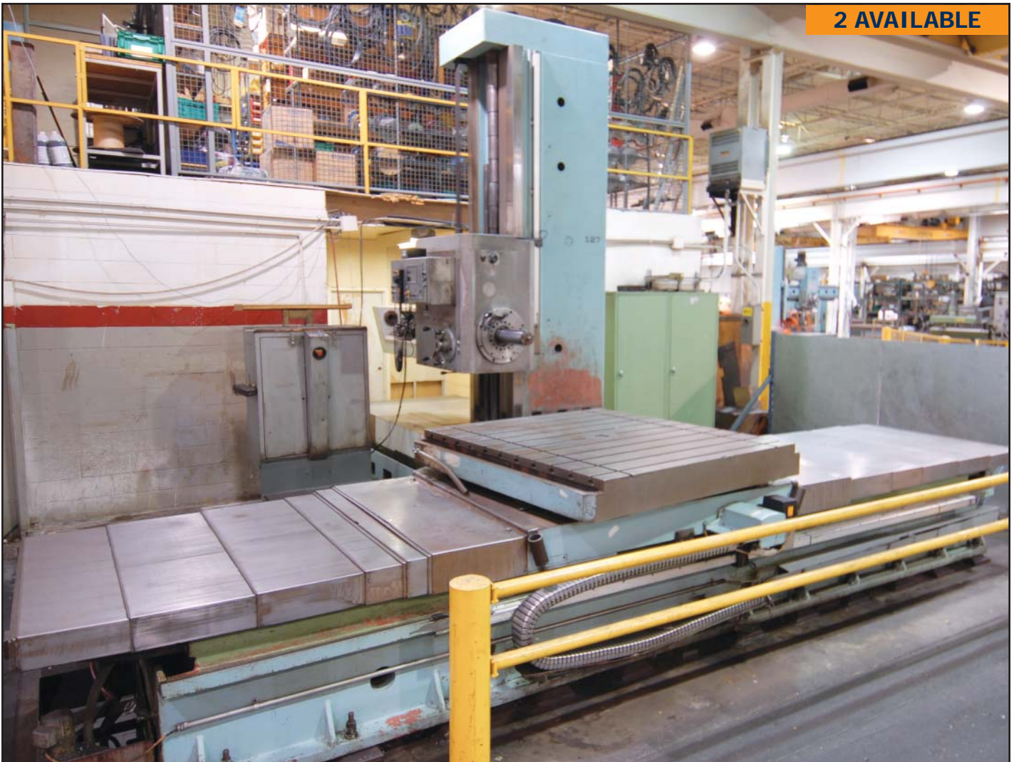
TOS WHN138A 5" table type horizontal boring mill
