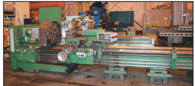
TOS SN63B gap bed engine lathe
