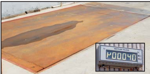
METTLER TOLEDO JAGJTGA 40 ton truck scale
