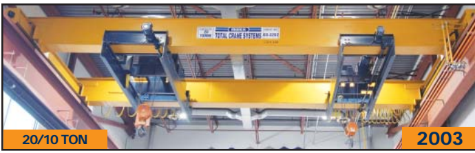
20/10 TON 2003 MUNCK 20/10 ton double girder top running bridge crane
