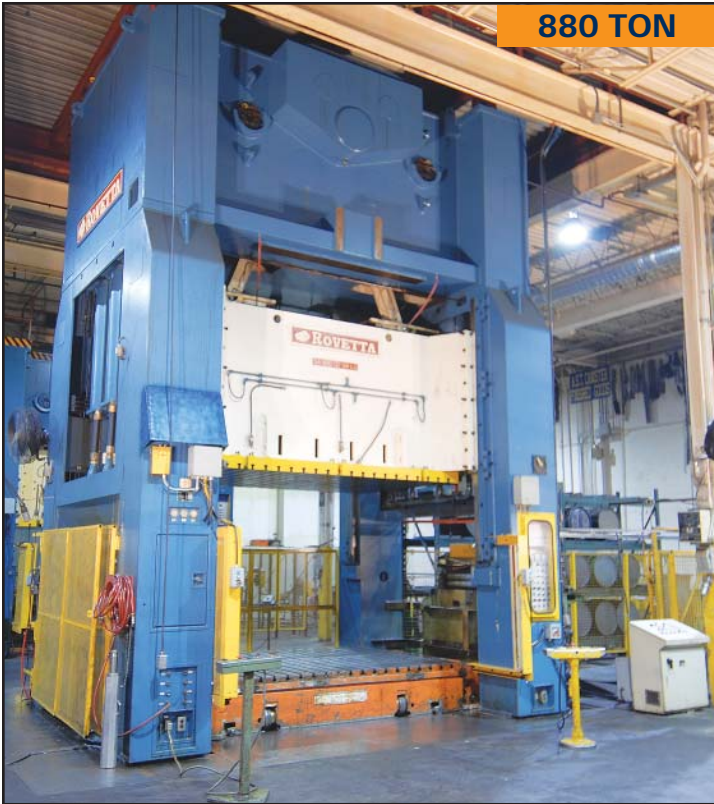
ROVETTA S4-880-132-84-LO straight side 4 point press
