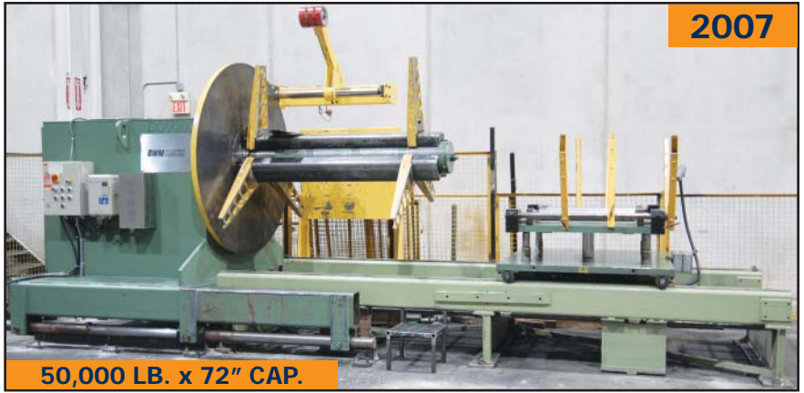
BARRIE WELDING & MACHINE U72-50-11-2007 mandrel type, traveling uncoiler
