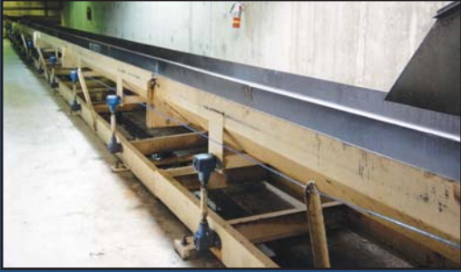
MAYFRAN scrap removal system with shuffle drive
