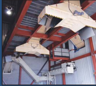
MAYFRAN scrap removal system with shuffle drive
