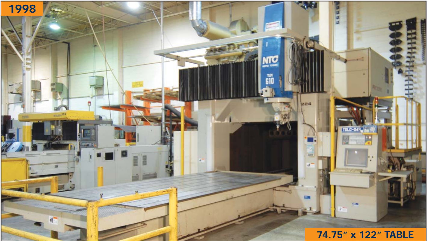
NTC TLM-610CWST 5 axis 2200 watt CNC laser
