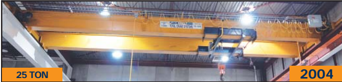
25 TON 2004 MUNCK 25 ton double girder top running bridge crane
