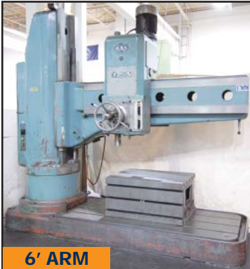
MAS VR6A way type radial arm drill
