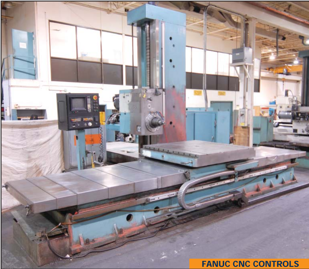
TOS WHN138C 5" CNC table type horizontal boring mill
