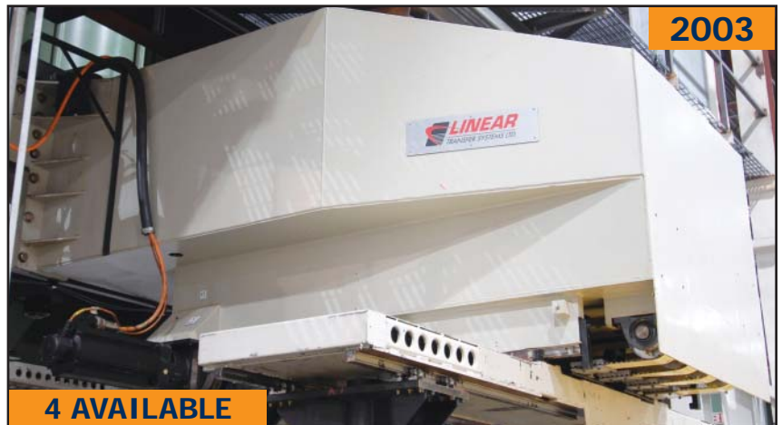
LINEAR TRANSFER SYSTEM LTS TITAN SERIES, 3-axis through the window, side mounted transfer system
