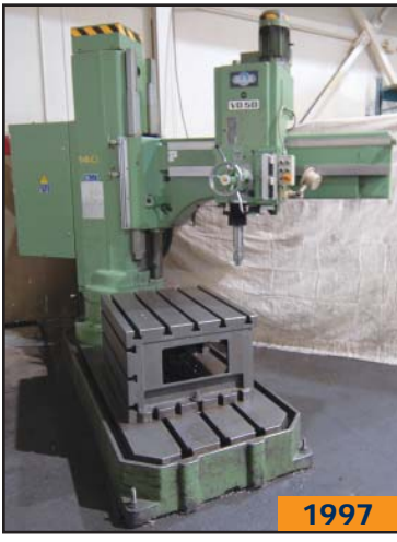
MAS V050 5' way type radial arm drill
