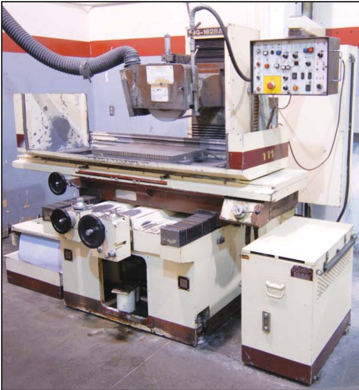
CHEVALIER FSG-1628AD hydraulic surface grinder
