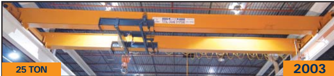
25 TON 2003 MUNCK 25 ton double girder top running bridge crane
