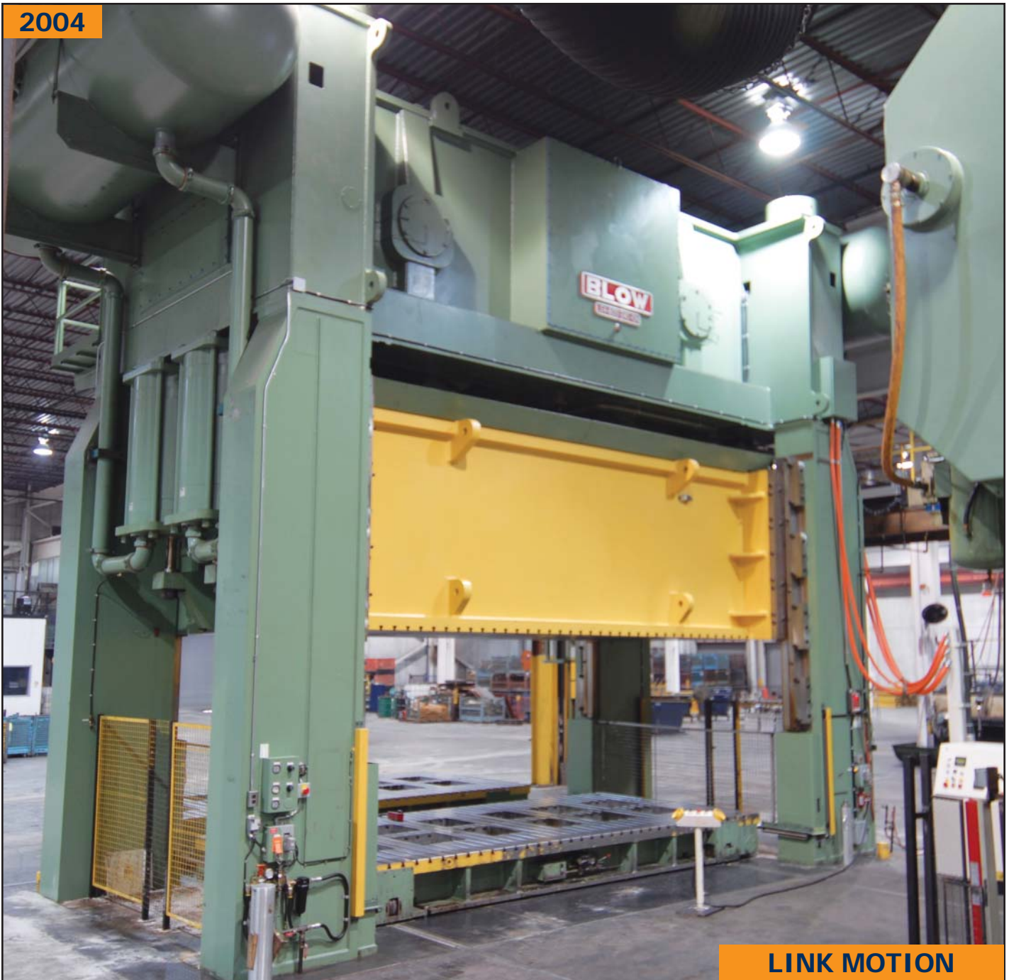
BLOW LE4-1600-240-108, straight side 4 point link motion press
