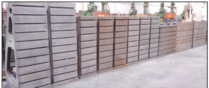
Partial view of angle plates
