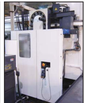
View of 38 station ATC
