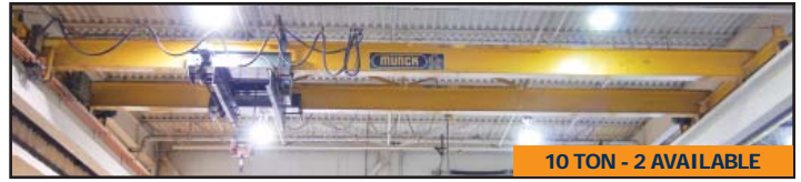
10 TON - 2 AVAILABLE MUNCK 10 ton double girder underslung bridge crane
