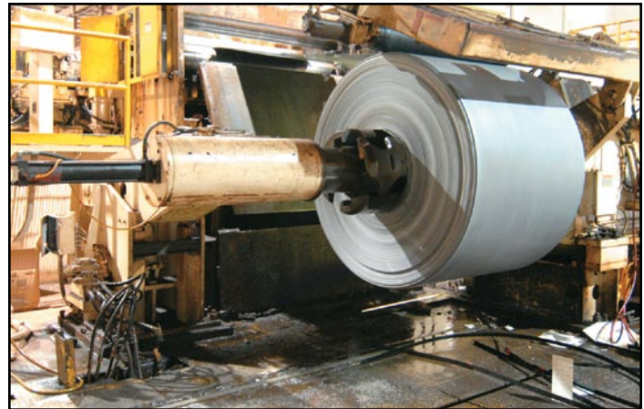
Uncoiler with hold-down roll, outboard bearing, edge guide unit, peeler, entry pinch rolls 3 roll breaker
