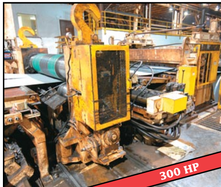
Entry crop shear, roller scrap conveyor, traversing slitter head
