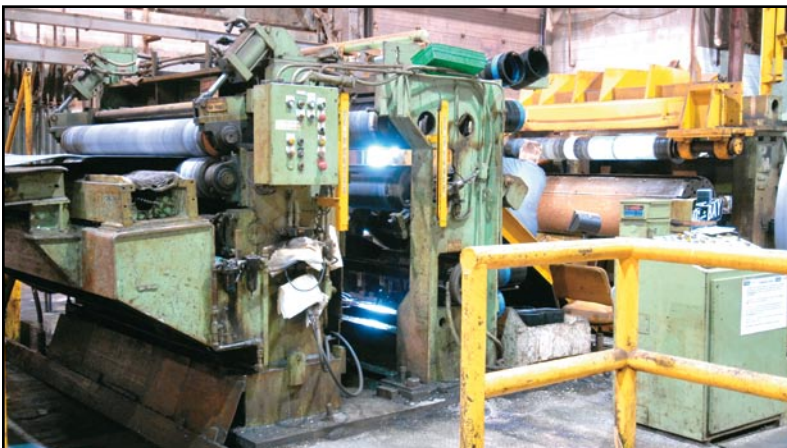
Pinch rolls, side guides, slitter, exit deflector rolls, thread table, edge guide unit, overarm separator, recoiler
