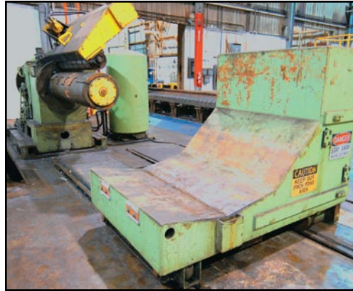
Floor mounted entry coil car, uncoiler with hold-down roll
