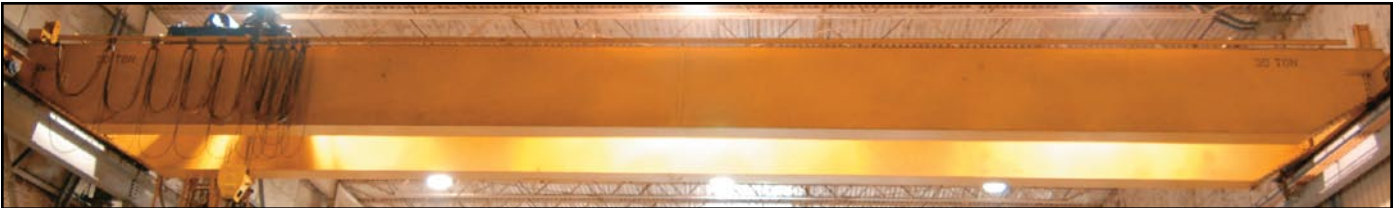
PROGRESSIVE 30 ton bridge crane
