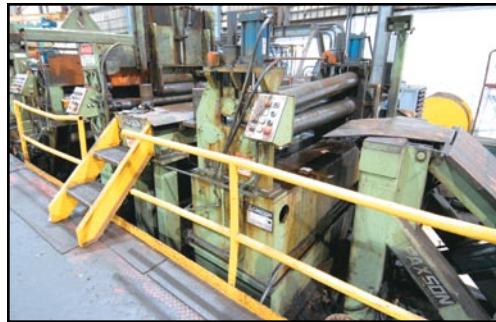
Entry pinch rolls, inspection table, entry crop shear, roller scrap conveyor, slitter pinch rolls
