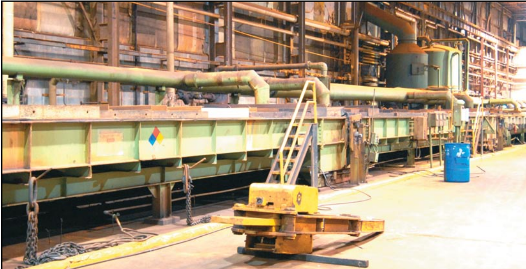
3 tray pickle section, 4 stage rinse section
