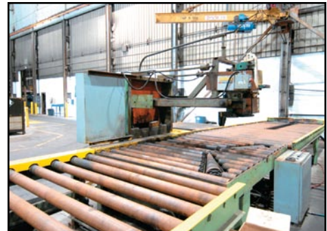
SIGNODE slit coil banding line
