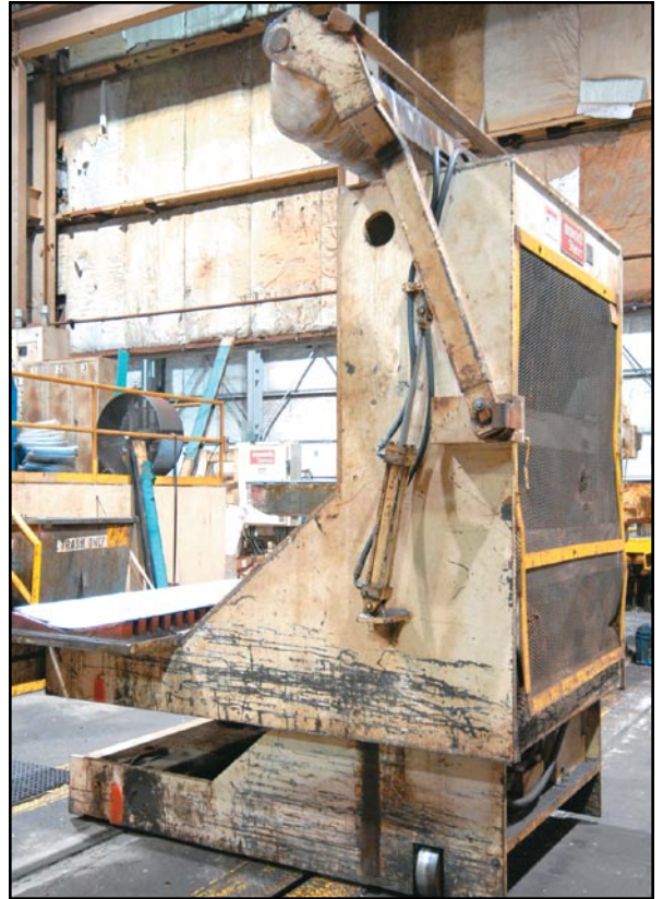
Floor mounted exit coil car
