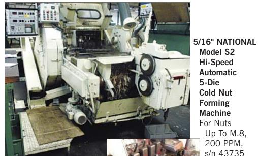
Model S2 Hi-Speed **Automatic** 5-Die **Cold Nut Forming** Machine For Nuts Up To M.8,
