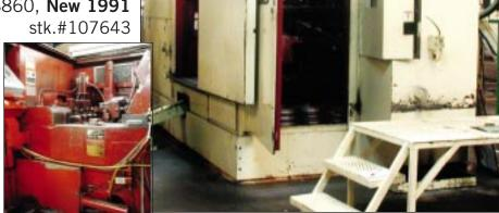
NATIONAL Model 124 **High Speed Automatic** 4-Die Cold Nut Former For Nuts Up To M.12, At 250 PPM,
