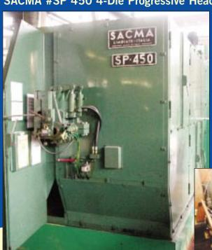
2000 Kn Heading Load, 4 Dies. 19mm Cutoff Dia... 165mm max. Cutoff, 120mm Die KO, 43.5mm Punch KO, 160 PPM, 75 HP, New 1988
