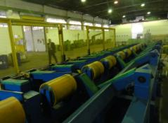
SCHUMAG KZ RP I COMBINED DRAWING MACHINE Draw sections: 6mm -10mm Round; 8mm-10mm Souare: 5mm-11mm Hex.
