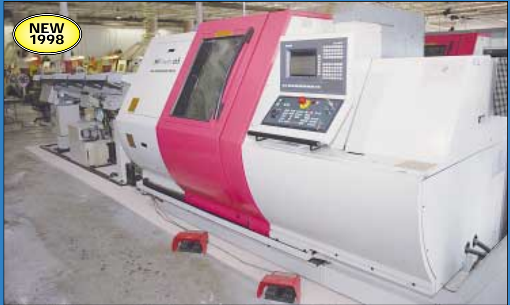
(2) Gildemeister Model MF Twin 65 Opposed Twin Spindle CNC Turning/Milling Centers
